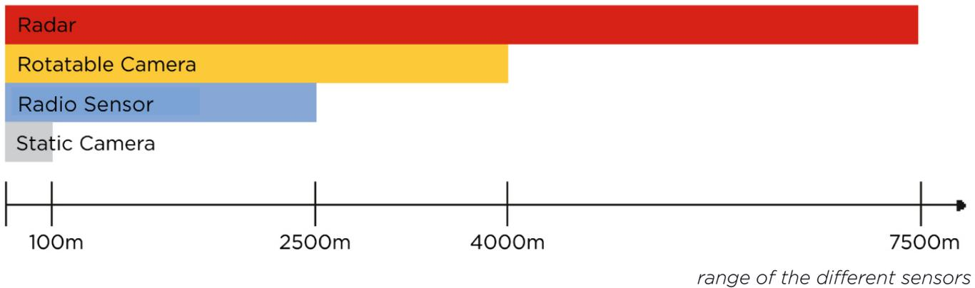
Example: A combination of radars, radio sensors and PTZ cameras for the optimal protection of an airport.
