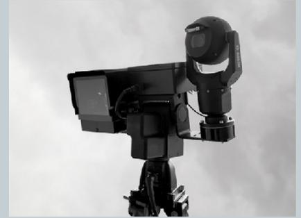
Optical sensors allow drone type and the carried payload to be identified.
