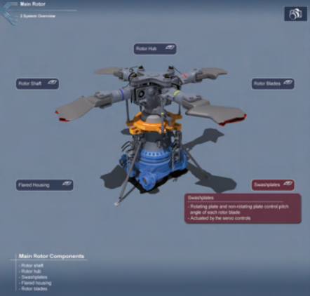
A typical courseware page explaining the main components of the rotor head assembly.
