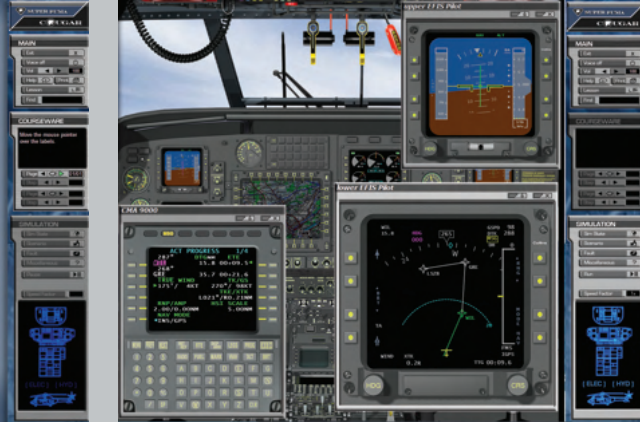
The simulator is about to capture a route controlled by the Automatic Flight Control System and the Flight Management System.
