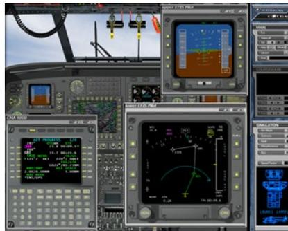
The simulator is about to capture a route controlled by the Automatic Flight Control System and the Flight Management System.
