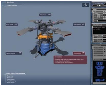
A typical courseware page explaining the main components of the rotor head assembly.
