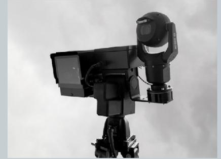
Optical sensors allow drone type and the carried payload to be identified.
